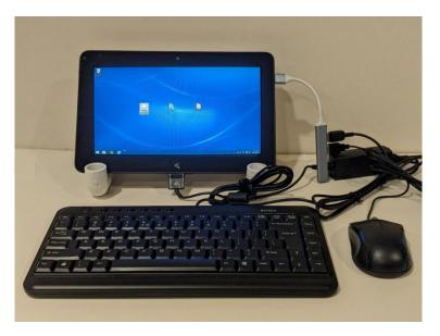
The computer is provided in a box to protect the screen during transport. A stand to hold the computer is included in the kit. Connect the power supply to the computer and then to an AC power outlet. Plug the USB expander into the USB port as shown. If the keyboard and mouse are not already plugged into the USB expander, do that now.
