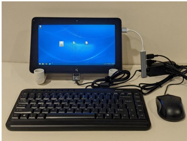
The computer is provided in a box to protect the screen during transport. A stand to hold the computer is included in the kit. Connect the power supply to the computer and then to an AC power outlet. Plug the USB expander into the USB port as shown. If the keyboard and mouse are not already plugged into the USB expander, do that now.
