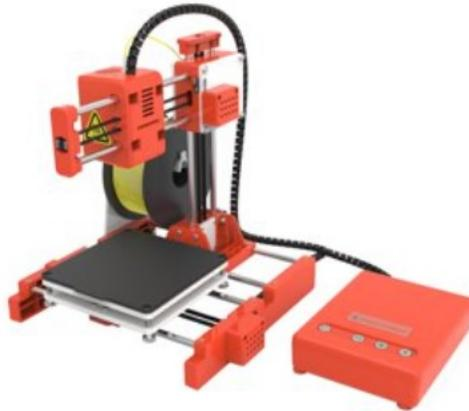
When originally purchased (Walmart.com; Amazon.com; etc.), the Easy3D Model X1 requires a small amount of assembly and there is the need to put the contents of the memory card on your computer and put the first test file to be printed on the memory card. Those steps have been taken for you, the memory card is in the control box with a file ready to print, and the 3D printer should be ready for the first print.
